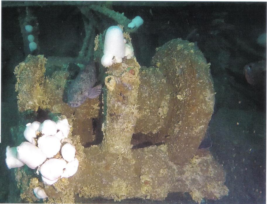
Steam steering gear of the *Conestoga* inside the shipwreck after falling through the main deck from its original position located below the pilot house. The steering gear served as “power steering” to assist the rotation of the large steering quadrant and rudder in the stern of the tug.
